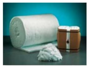
Ceramic fibers can be transformed into ropes, mats, felted paper, and even foams. (Photo courtesy of Unifrax<sup>©</sup>)
